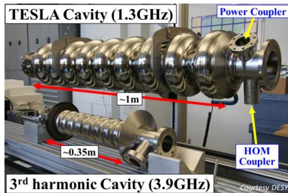
Superconducting accelerating cavities (Image credit: DESY)
