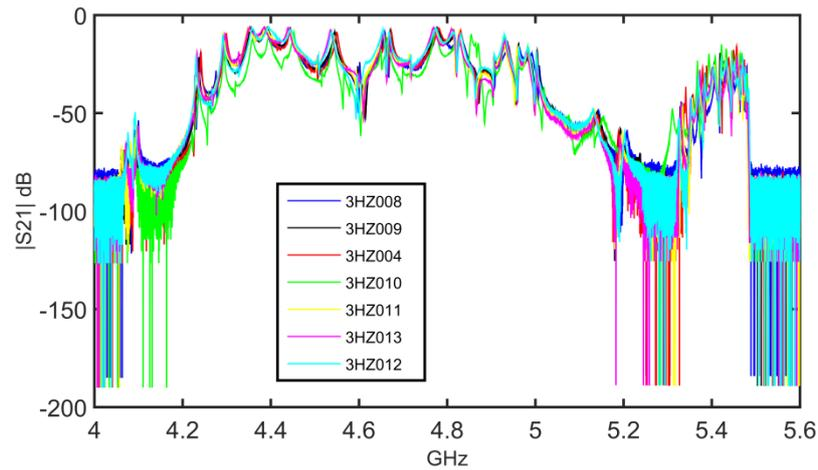
*Room temperature spectra of individual 3.9GHz cavities for the E-XFEL*
