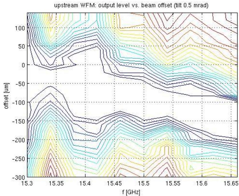
*Detecting structure tilts in the spectral density of a WFM signal*
