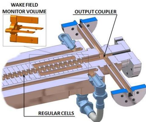
Down stream end of X band structure with wake field monitor pickup (Image credit: PSI)
