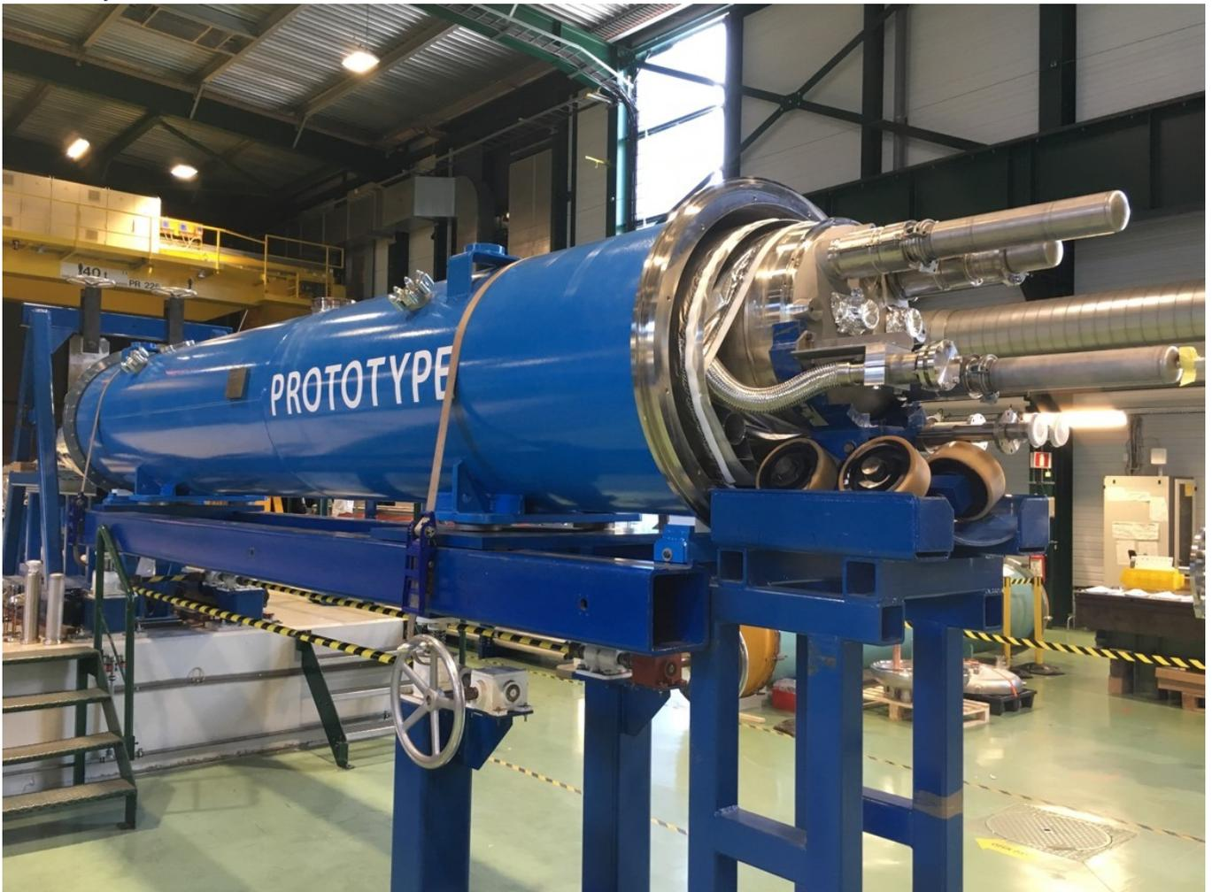
The construction of the 5.5-m long 11T dipole prototype was completed in May this year
