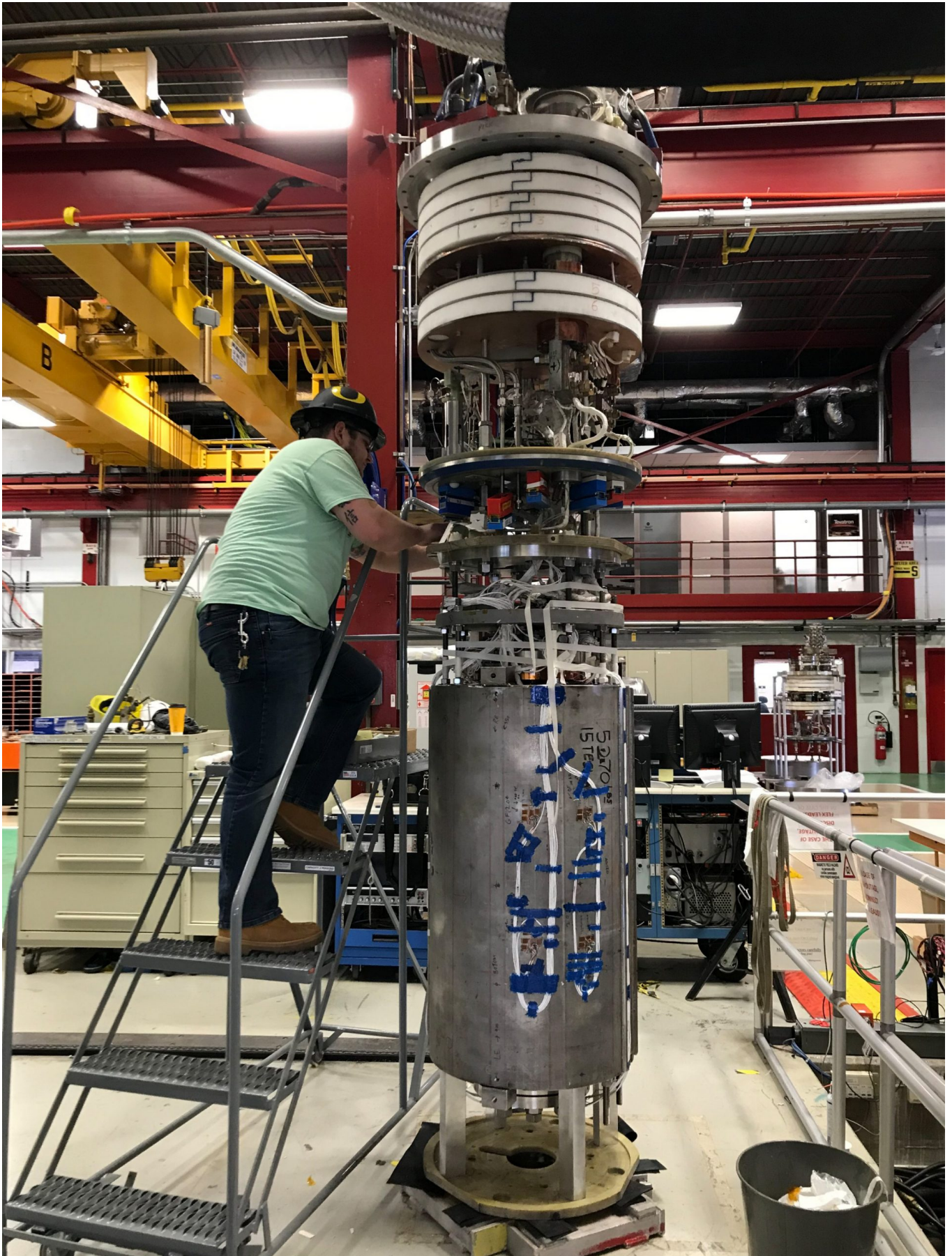
A member of the Fermilab magnet team prepares the demonstrator accelerator magnet for testing in March 2020. These tests are an important step toward meeting the requirements of a future hadron collider under discussion in the particle physics community. Photo: Alexander Zlobin
