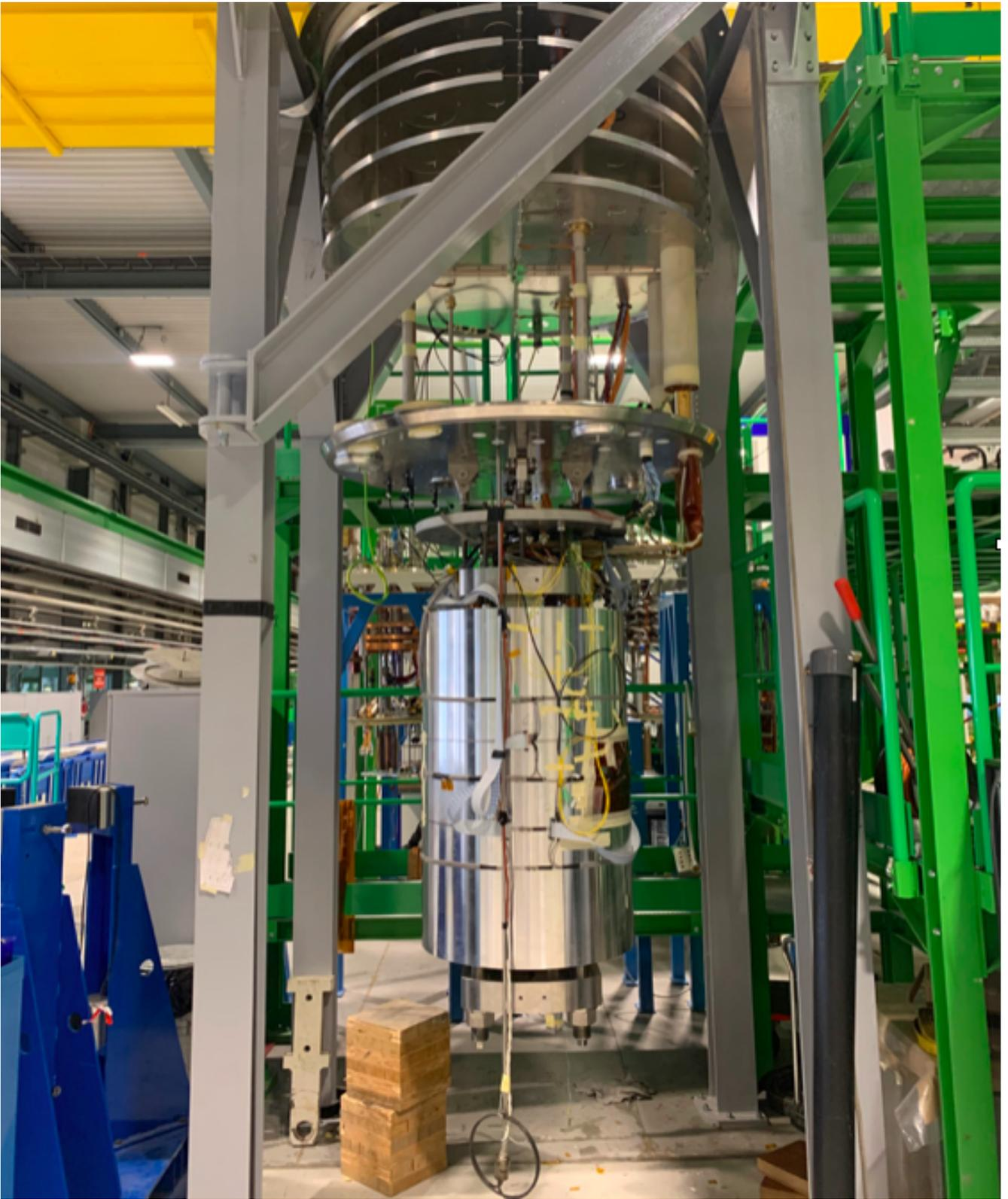
The enhanced Racetrack Model Coil (eRMC). (Image: CERN)
