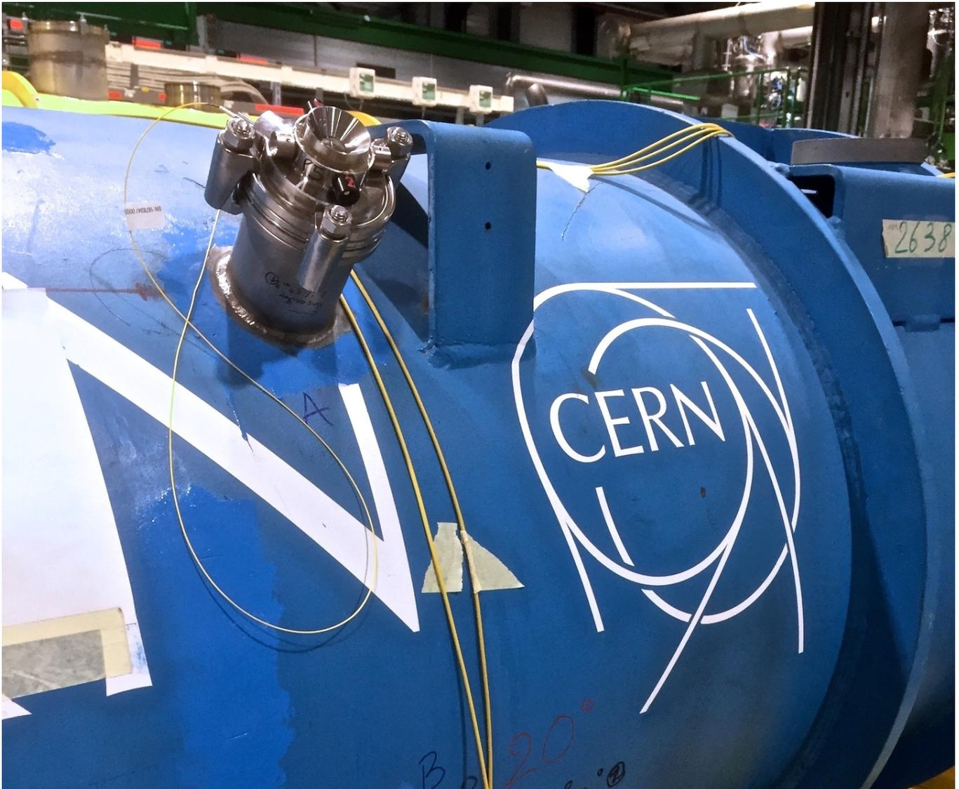
A cryostat can be equipped with 12 laser heads such as the ones seen here (the two devices connected to yellow cables). Facing each laser head is a reflective target (not seen), which is attached to a cold mass inside the cryostat (Image: CERN)
