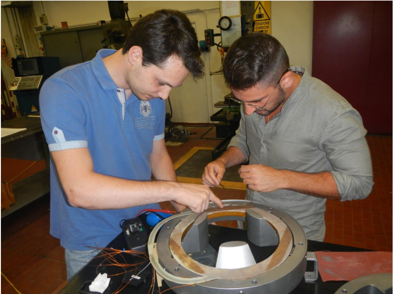
Figure 1: Assembly of the MgB 2 superconducting coils in the iron pole and yoke.
