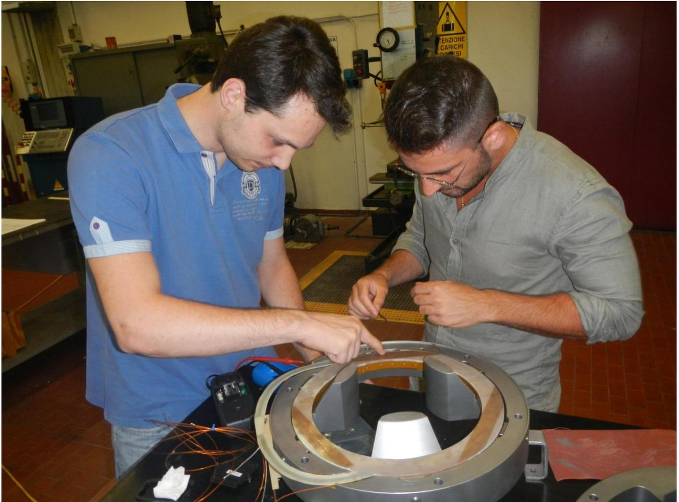
Figure 1: Assembly of the MgB<sub>2</sub> superconducting coils in the iron pole and yoke.
